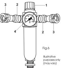
NOTE: Pressure Gauge (4). Pressure shown will differ by approximately 1 bar depending on whether the outlets are open/closed.
