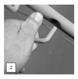
2.20 Insert the end of the cable in to the location hole on the lever (3).
