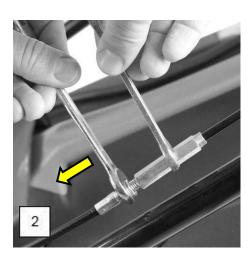
2.33 Wind the adjuster nut towards the main handlebar.
