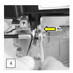
2.29 Check the cable adjustment has worked by starting the mower. If the mower still fails to start, re-adjust until the lawnmower starts.
