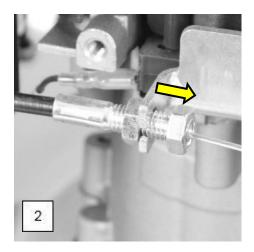
2.27 Move the adjustment nut towards the lock nut and continually check the cable tension at the lever (3).
