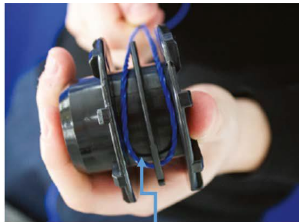
Place the looped end over the spool
