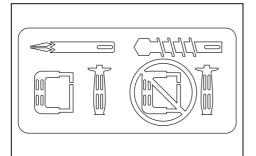
**ACAUTION:** Use the side handle only when chipping, scaling or demolishing. Do not use it when drilling in concrete, masonry, etc. The tool cannot be held properly with this side handle when drilling.
