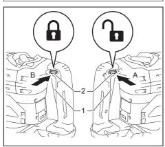
▶ 1. Switch trigger 2. Trigger-lock button
