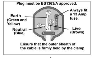
connected to the terminal which is marked E or \to roloured green.
