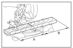
A) When you want to obtain the correct size on the left side of workpiece, shift the laser line to the left of the blade.
