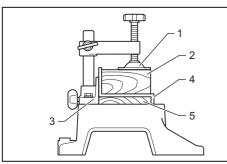
1. Vise 2. Spacer block 3. Guide fence 4. Aluminum extrusion 5. Spacer block When securing aluminum extrusions, use spacer blocks or pieces of scrap as shown in the figure to prevent deformation of the aluminum. Use a cutting lubricant when cutting the aluminum extrusion to prevent build-up of the aluminum material on the blade.
