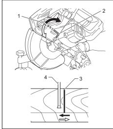
1. Range adjustment screw 2. Hex wrench 3. Laser line 4. Saw blade
