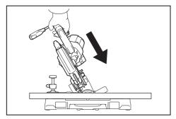
1. Loosen the lever and tilt the saw blade to set the bevel angle (Refer to the previously covered "Adjusting the bevel angle"). Be sure to retighten the lever firmly to secure the selected bevel angle safely.
