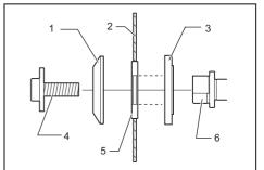
Outer flange 2. Saw blade 3. Inner flange 4. Hex socket bolt (left-handed) 5. Ring 6. Spindle
