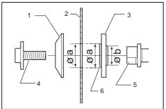
Outer flange 2. Saw blade 3. Inner flange 4. Hex socket bolt (left-handed) 5. Spindle 6. Blade mounting part
