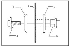
Outer flange 2. Saw blade 3. Inner flange 4. Hex socket bolt (left-handed) 5. Spindle
