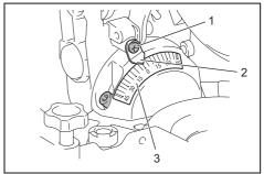
1. Screw 2. Pointer 3. Bevel scale
