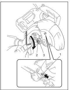
▶ 1. Shaft lock 2. Hex socket bolt 3. Outer flange
