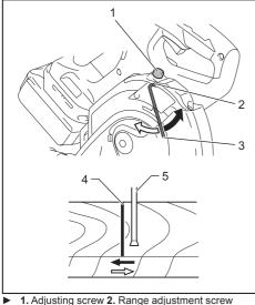
1. Adjusting screw 2. Range adjustment screw
