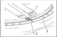
1. Screw 2. Miter scale 3. Pointer
