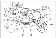
1. Fixing screw 2. Turn base 3. Miter scale
