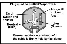
connected to the terminal which is marked E or  $\neq$  or coloured green.
