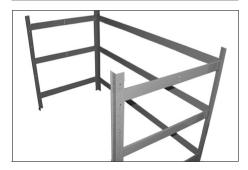
Connect the support beams (E) to the long beams (C) by bending the flexible tabs to 90 degrees and slotting them into place as shown. Finally bend the tabs back 180 degrees to lock in place.
