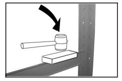
Use the short beams (D) to connect the front and rear posts together.
