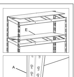
We recommend that the racking be secured to an adjacent wall using typical wall insert plugs and screws (not supplied), aligned with the assembly slots in the posts.
