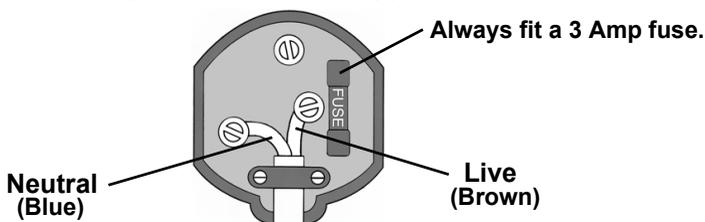
**Ensure that the outer sheath of the cable is firmly held by the clamp**
