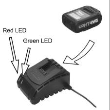
The battery pack should slide in easily. If it is not to be fitted immediately, ensure that the metal contacts are protected to avoid the possibility of a short circuit which would cause battery damage. For maximum battery life, we recommend that you maintain the battery in a fully charged state.
