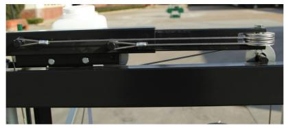
Install the cables to the pulleys as shown above.
