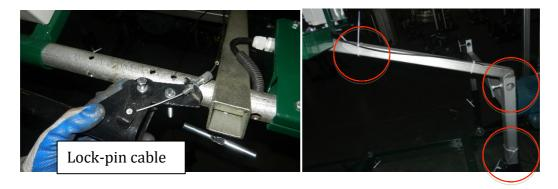
Connect the lock-pin cable to the guiding-wheel-locking-handle. Fix the cable to the L- handle with the 3 nylon ties. To make sure the engine can run at the highest speed when the throttle handle is fully pushed down. To make sure the guiding wheel can running smoothly when the guiding wheel locking handle is pushed down.
