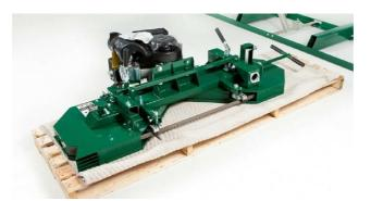
Place a moving blanket on the shipping pallet that the sawmill crate was strapped to. The blanket will prevent the blade guard covers from becoming scratched. Using a **minimum of two people** or a mechanical advantage system, remove the head assembly from the sawmill crate and place face down on the blanket. The head assembly is very heavy, proper technique must be used to avoid injury or damage.
