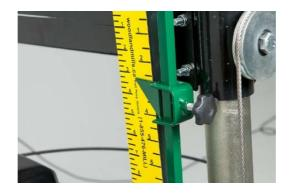
Slide the scale indicator over the square rod and tighten.
