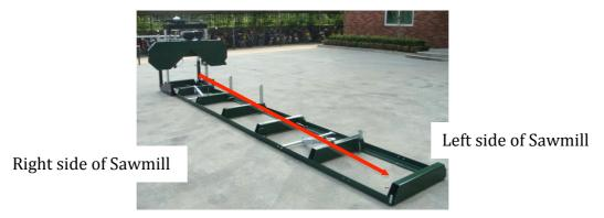
Always cut in the direction shown above. The log clamp should always be on the right side of the log and the log supports should always be on the left. Failure to cut in this direction can cause the log to come lose and possibly even cause damage or injury.
