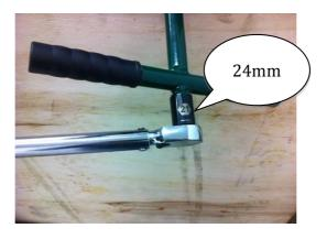
Use a 24mm socket on a torque wrench to tighten the "T" handle to 25 N.M torque. See above image.
