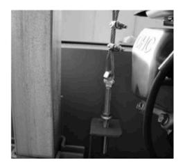
Attach the cable bolts to the brackets on the sawmill head as shown above. It is ideal to lower the sawmill head all the way down to the deck. Once this is done, adjust the two bolts so that the sawmill head is level to the track cross supports. See next page for further details on this set up.
