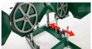
Remove the tension in the blade by turning the "T" handle in the counter-clockwise direction and then open the blade guard cover. The blade should now be loose and free to pull straight out the front.
