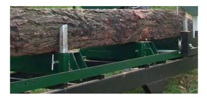
Push the log/cant to the Supports and make sure there is no space left between the log/cant and the Supports. (For supports use, Refer to page 11.)
