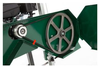
To check the belt tension, with a tension meter, deflect the belt up and down with 60N force. There should be no more than 5-6mm of deflection in both directions. If the belt deflects more than this, it will need to be tightened as described below.
