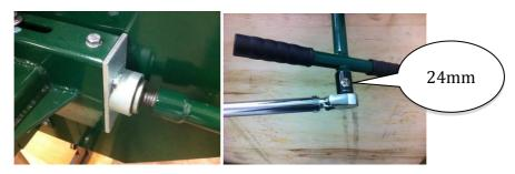
Add waterproof grease to the threads of the blade tension "T" handle and to the washer face that it meets before use. USA a 24mm socket on a torque wrench to tighten the "T" handle to 25 N.M torque to achieve proper blade tension. See above right image.
