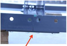
Attach track cross supports to "L" channel with the provided nuts & bolts. The joining plate (assembled under two rails) is used at the seam joint to join the two sections together (shown in right images). Ensure to only hand tighten at this stage. The bolts will be fully tightened once the head assembly is free to roll on the tracks and provide the correct track width.
