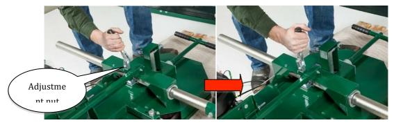
Lock the cam handles on both the round and square post to prevent the head from moving when it is stood up in the coming steps. Ensure that when activating the cam handles, the clamps securely lock on the round and square vertical post. If they don't, a 13mm wrench will need to be used to tighten the adjustment nut. This will allow the clamps to lock on the post better.
