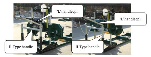
Insert the H-type handle piece into the carriage vertical posts. Insert the "L" handle to the right vertical post. Adjust the height of the handles and lock them with the T-bolts. Please refer the above picture.
