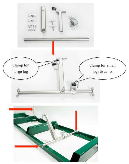
Attach log dog assembly to track as shown above with the 4 nuts and bolts provided. Note that there are various locations along the track where this assembly can be bolted. Depending on how many track sections are being used, select a log clamp position that will secure the log firmly against the log supports.
