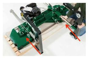
Insert vertical post assemblies into corresponding locations in head assembly as shown above.
