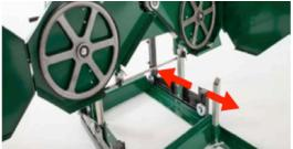
Remove the tension in the blade by turning the "T" handle in the counter-clockwise direction and then open the blade guard cover. The blade should now be loose and free to pull straight out the front. The new blade can now be installed, guards closed and proper blade tension set.
