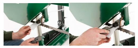
Using a piece of paper in between the blade and blade guide blocks, tighten the allen key bolts.
