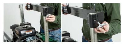
Slide the top cross support over the round post and insert the pulley, collar and bolt assembly into the hole.
