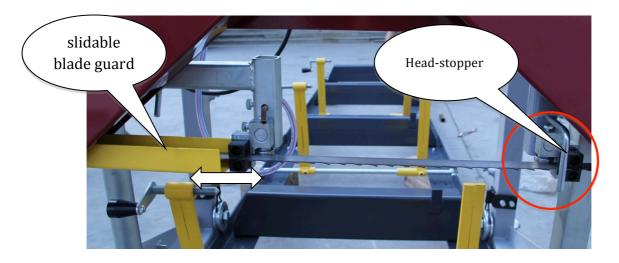
Loose two T bolts on the tube showed above in the red circle, and then slid the blade guard left/right to adjust the blade length for cutting.
