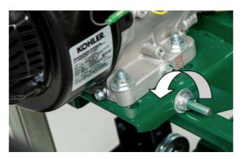
Now that the engine is free to slide on the engine mounting plate, turn the 16mm nut on the horizontal stud in the counter-clockwise direction. This will allow the engine to move and will also take the tension off of the belt. The old belt can be removed and the new belt can be installed. Tension the new belt and refer to the **BELT TENSION** instructions described in the sawmill set up section of the manual.
