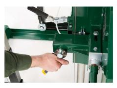
Loosen the tracking alignment locking nut.
