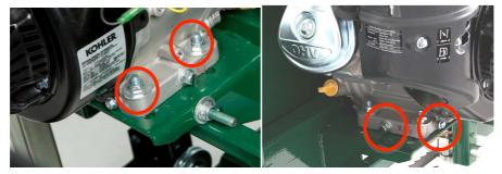
To change the drive side belt, loosen the four bolts that secure the engine to the engine mount using a 16mm wrench.
