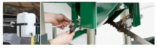
Put the lube tank to the bracket. Insert the lube tank line through the hole in the bottom of the saw head as shown above. Use a 16mm socket to secure the copper end in position. Do not over tighten or crush the copper end.
