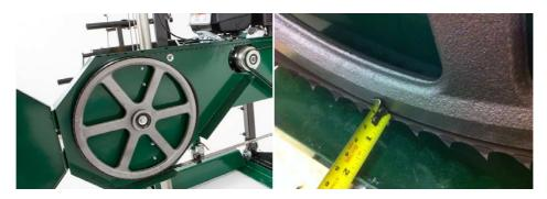
Wearing gloves, spin the bandwheel with your hand and observe how the blade has changed tracking. Measure the distance again and repeat the above step to further compensate if required. The ideal measurement is 9.5mm.
