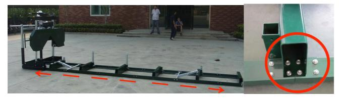
Push the saw head up and down the track system to ensure that the width of the track allows for the saw head to move freely. If it binds, the "L" rails will need to be set further or closer together to achieve a consistent width along the entire track system. Once the desired width is achieved, all nuts and bolts can be tightened to the log bunks as shown in above right image using a 16mm socket.
