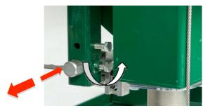
Loosen the blade guide assembly bolt with a 16mm socket. The round shaft should now be free to slide rearward and out of the way. Perform this step on both guide assemblies. This will ensure that the guide bearings do not influence tracking of the blade while adjusting.
