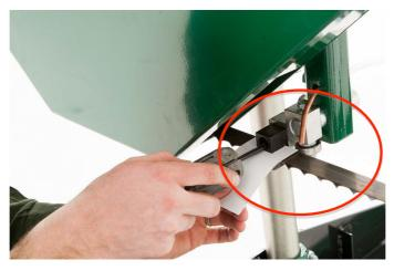
Using a 6mm allen key, loosen the blade guide blocks on both the left and right sides. They should be free to slide up and down.
