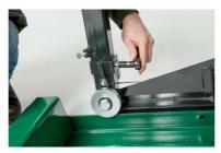
Attach the four track sweepers to the frame so that the steel brush reaches the bottom of the groove in the carriage wheels. Use a 13mm socket to fasten.
