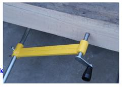
\*\*\*Do not forget to lock the log/cant again before cutting.
