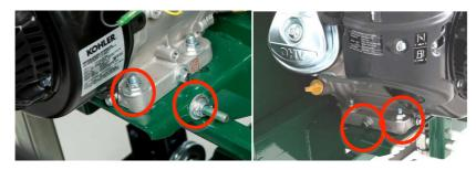
To tighten the drive belt, start by loosening the four bolts that secure the engine to the engine mount using a 16mm wrench.
