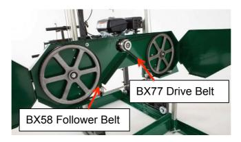
There are two rubber "V" belts on the sawmill and they should be replaced as a set. It is not advised to replace individual belts separately. It is recommended to to use a BX77 cogged belt for the drive side and a BX58 follower belt.
