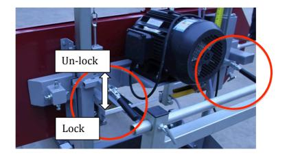
Loose two lock handles of the Saw-head.
