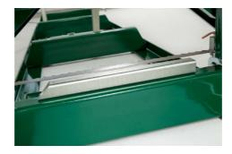
Using a tape measure, take a measurement from the blade to the top of the log bunk on both the left and right side. The distance should be equal on both sides. If it isn't, you need to adjust the cable bolts (shown on page 13) up or down to raise or lower the head on one side until themeasurement is consistent on both sides.
