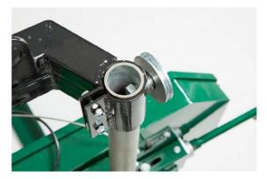
Install the nut on the inside of the round post to secure the pulley. Using a 16mm wrench to hold the nut, tighten the bolt.
