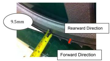
The blade should run with the same tooth to bandwheel face distance on both sides. 9.5mm is ideal. Measure the distance from the tip of the blade tooth to the front face of the bandwheel on both sides. If an adjustment on either side is required, the below steps will detail this procedure.
