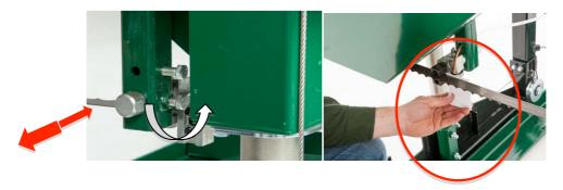
Loosen the blade guide assembly bolt with a 16mm socket. The round shaft should now be free to slide back and forth. Position it so that there is a paper width gap between the bearing and the back of blade. Tighten bolt against the flat on the shaft to secure assembly back in position.
