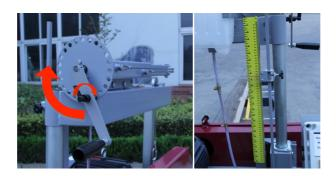
Turning the Crank to adjust the height of the cutting head of the Sawmill to reach suitable height.
