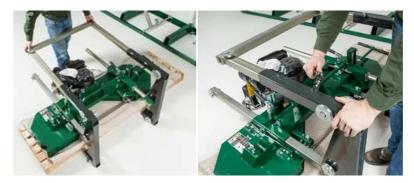
Insert the rear square frame into the carriage base until it bottoms out on the pulley bolts. Tighten the four 16mm bolts (shown in right image) to secure it in place.
