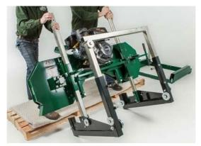
With one person on each post, stand the head assembly up on the wheels as shown above. Again, using a **minimum of two people**, set the saw head assembly on the track system ensuring the carriage wheel grooves rest on the "L" rails. The square vertical post should be on the same side as the log supports.
