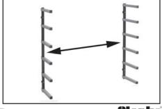
Position the spacers between the mounting holes and the wall, and fasten to the wall using suitable fixings.
