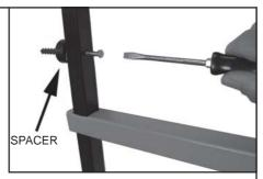
Note: You will need to provide screws and wall plugs of the correct type, able to adequtely support the weight you intend to place on the rack.
