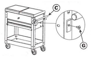
The handle can be attached to either side using two screws.
