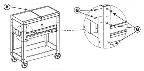
Turn the upper tray upside down on a soft, smooth surface. Turn the bottom tray upside down and attach all four legs. Firmly tighten all the screws and turn the trolley upright.
