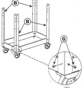
Attach the legs to the bottom tray using two screws per leg. Only tighten to a snug fit at this stage.
