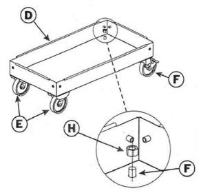
Attach the wheels to the bottom tray using 4 nuts and tighten firmly.
