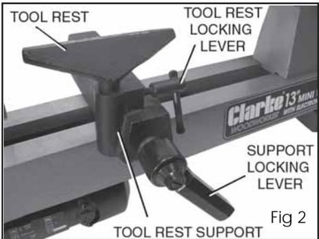
The position of the support will be adjusted to suit the workpiece.
