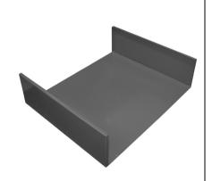
17. Fold up the ends of the drawer base (5) along the creases as shown.
