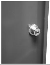
12. Insert the lock barrel with the green window at the top through the door and secure using the locknut as shown.
