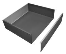
18. Fit the drawer sides (6) and secure to the drawer base (5) using the small machine screws and nuts to secure.
