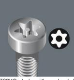
TORX® tools with a borehole prevent the unauthorised unfastening of safety screws. The screws contain a pin that protrudes into the drive profile so that "normal" TORX® tools cannot be used. This pin fits into the borehole of TORX® BO tools allowing safety screws to be unfastened.
