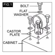
the washer, castor plate and into the unit, Tighten with a spanner. Repeat for the remaining bolts and castors.
