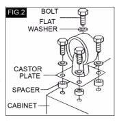
plate on top of spacers and insert the bolts through castor plate, spacers and threaded holes of storage unit. Tighten with a spanner. Repeat for all remaining bolts and castors.
