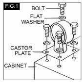
washer, castor plate and into Storage Unit, Tighten with spanner. Repeat for remaining bolts and castors.
