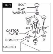
Line up castor plate on top of spacers and insert bolts through castor plate, spacers and threaded holes of Storage Unit. Tighten with spanner. Repeat for remaining bolts and castors.
