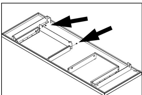
downwards using two M8 bolts with each leg, ensuring a flat washer is used with the nut. Nip up the nuts - DO NOT fully tighten.
