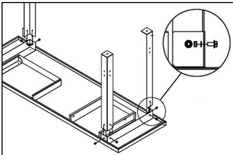
4. With the help of an assistant, position the shelf between the legs, and bolt it to the legs using M8 bolts with nuts and flat washers. DO NOT fully tighten the nuts.
