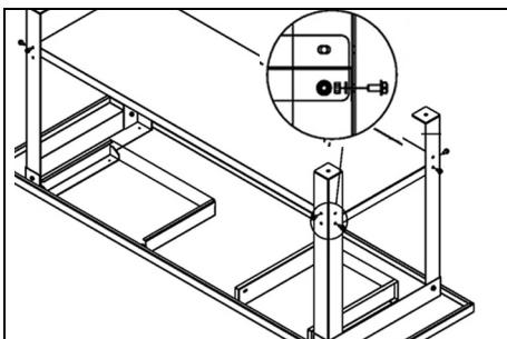
5. Turn the workbench on to its feet and shake it vigorously to ensure it is completely stable and resting evenly on all four legs, then fully tighten all nuts.
