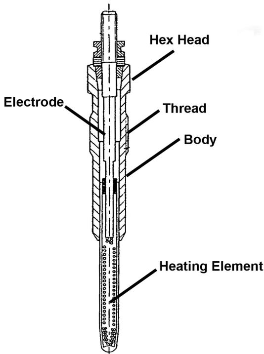
**Fig.3-Glow Plug with Electrode withdrawn**
